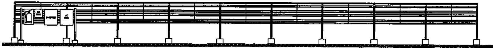
REAR ELEVATION WITH FIRE EXTINGUISHER, DC BOX, INVERTER & AC BOX SubSPV-BDC-17.011 SCALE NTS
